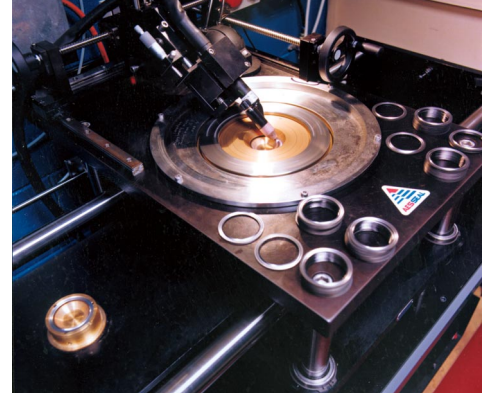
CNC inside diameter bellows welding operation.
